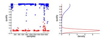
Fig. 5. Quality Measure for angle measures (left, keys like Fig. 3) for test set 3; Gaussian density functions for accurate (top) and not accurate (bottom) angle measures (right)
