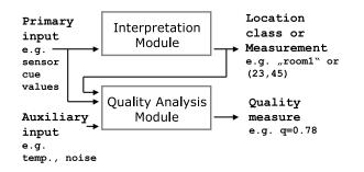
Fig. 2. Schematics of a general system for location measurement or classification with a parallel system for quality analysis.
