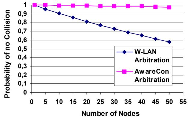
Figure 6. Probability of no Collisions for W-LAN and AwareCon arbitration
